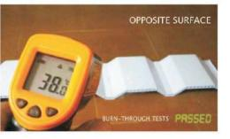
After burned for 21 seconds at + 370°C, flames were extinguished and the opposite surface were nt burnt at all. DELTA is fireproof and fire-retardant property that prevent fire to spread, so it highly recomended for your
