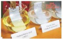
DELTA are chemical resistant for following substance: HCl (Hydrochloric Acid ), Caustic Soda (Sodium Hydroxide ), Paint Thinner, Benzene and Salt Water. So **DELTA** is safe for industries that use chemicals.
